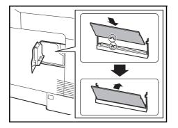
**5** With the memory connection terminal pointing toward the socket, align the cut-out part with the socket terminal and insert directly in at an angle.
